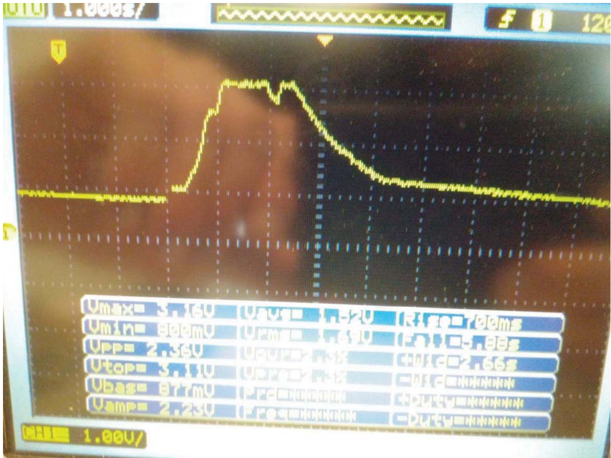
Figure 44. Voltage over time measured at the GND and the VOUT pads of the LTC3105 board with a TYP 20G-150 motor connected to a rectifier board used to supply power. The voltage is measured over a 100 \mu F capacitor.
