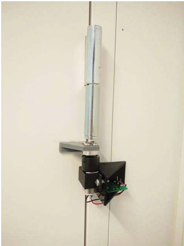
Figure 36. Test set-up of TYP 20G-150 motor with a LTC3588-1 power management board.
